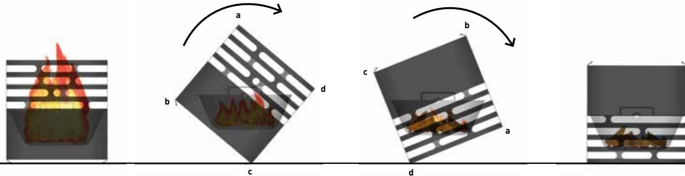
**!** IMPORTANT! CUBE may only be tilted over the edges with foot (b and c) resp. the edges with handle (a and d), e.g. CUBE may only be tilted over the edges having the same alignment as the bearing axle of the firebowl. ATTENTION! If not observed, the firebowl will turn, not remain in balance and the content of the firebowl will be dumped.
